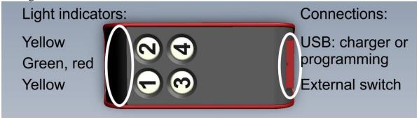
If **page 2 is be enabled** the Pico4 and Pico8 use the lower left key as a page-select key. In this case it will not transmit any IR-signals. Pico4 will have a maximum of 6 channels and Pico8 will have a maximum of 14 channels if page 2 is enabled. Pico16 has a dedicated page select key.
