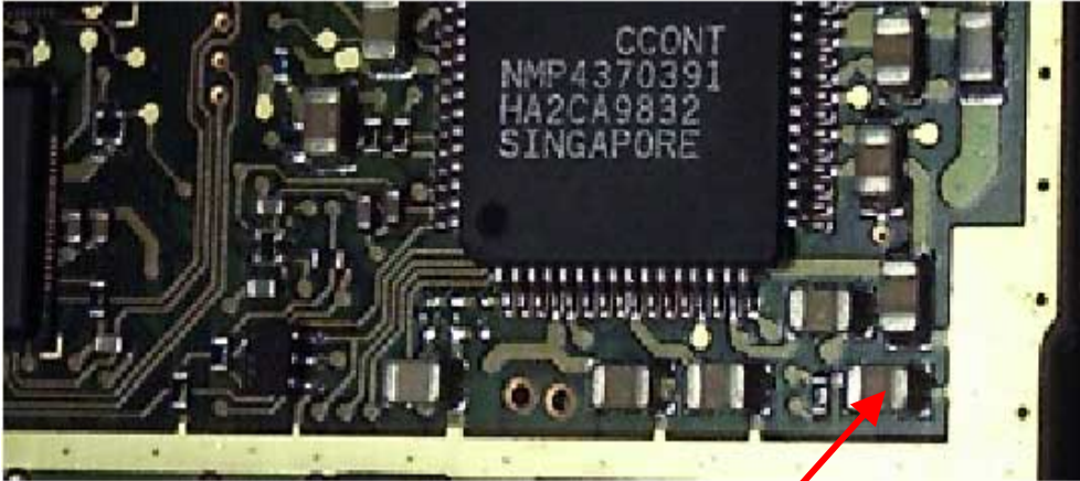
Broken or cold joint
