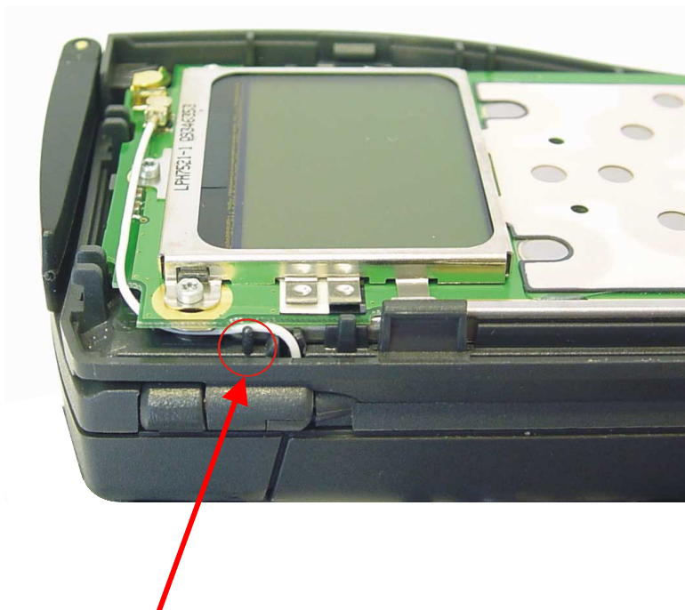
Cable routed behind the guidance rib
