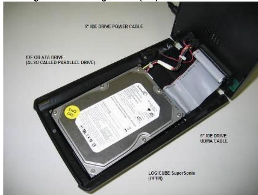
**Figure 3. Connecting a PATA (IDE) Target Drive**
