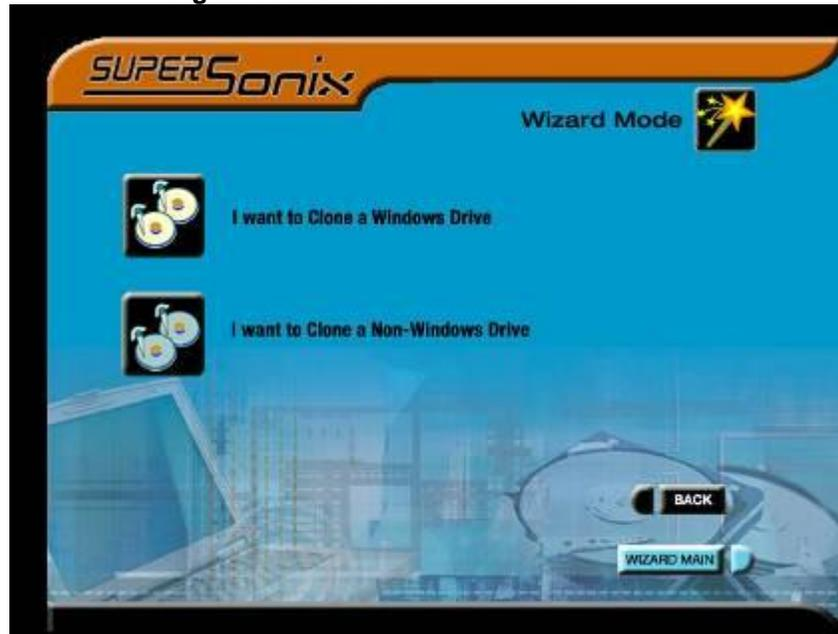
Irrespective of which selection is made (Windows Drive or Non-Windows Drive) the user will be prompted to select the location of the Master Drive. See Figure 8 for an example of what you can expect to see on the display.
