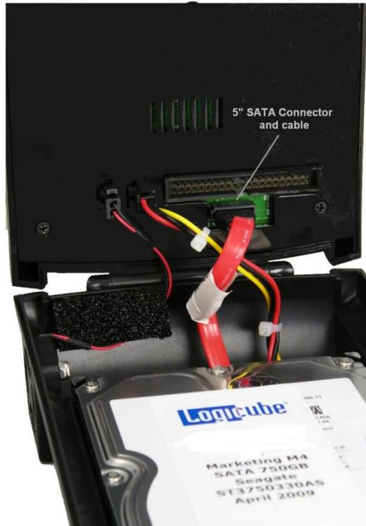
Figure 5. Connecting a SATA Target Drive.
