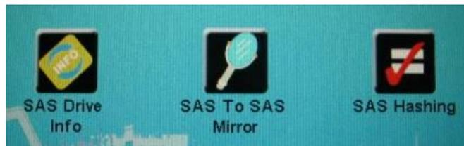
3. You can perform a drive info check to verify that the SuperSonix recognizes either of the SAS drives connected through the SAS adapter. Press the SAS Drive Info icon and
