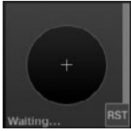
Figure 7.8 Scope view displays timecode clarity as well as potential complications. Click the RST button to begin the Calibration process.
