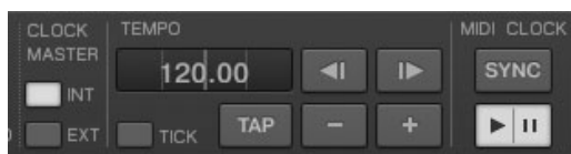
Figure 8.26 Use this panel to control Traktor's MIDI Clock playback performance.
