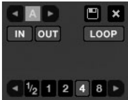
Figure 9.38 SSL's performance-focused looping controls.
