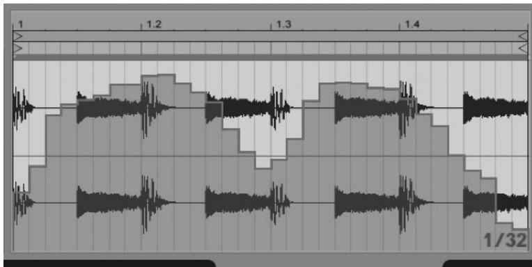
Figure 11.13 Use breakpoint envelopes to automate Live's parameter behaviors.
