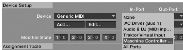
Figure 8.2 All connected MIDI-capable gear should show up within the In-Ports menu.
