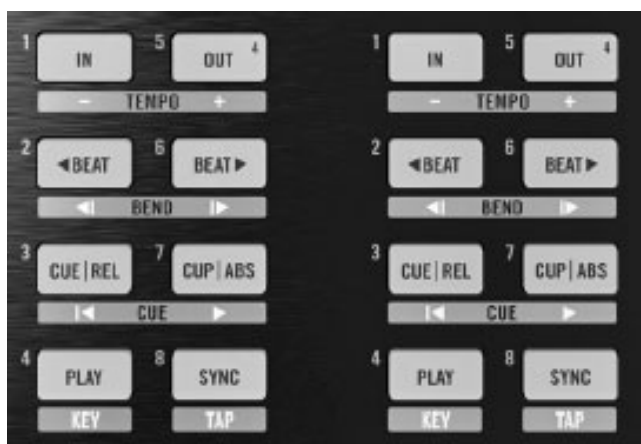
Figure 8.16 Use the X1's Transport section to control Traktor's playback behaviors.
