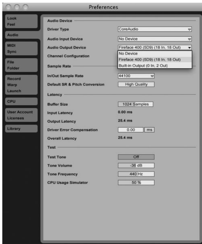
Figure 10.1 Choose your audio interface from the Audio Output Device drop-down menu.
