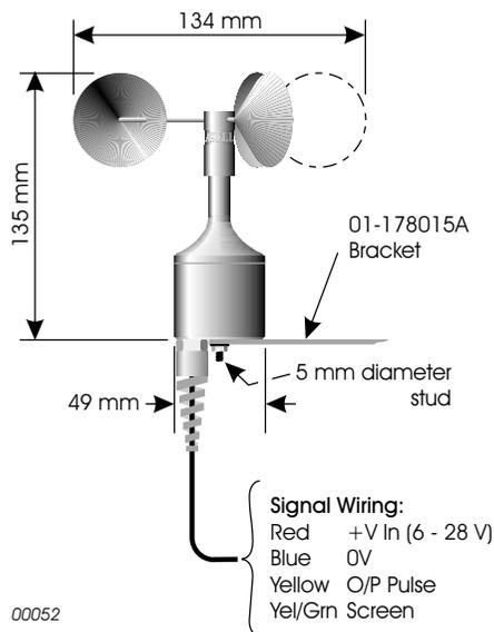
Figure 1: Anemometer wind speed sensor
