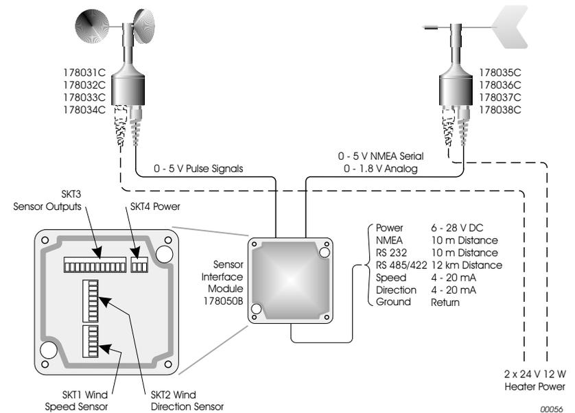
Figure 5: Connections for the anemometer and windvane
