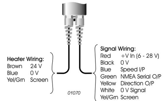
Figure 4: Connections for Wind-vane versions with heaters
