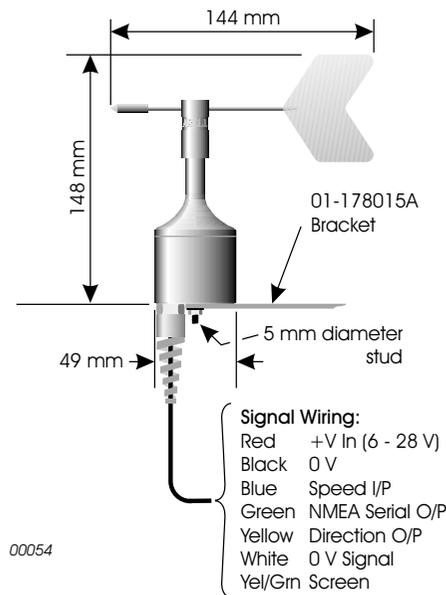
Figure 3: Wind-vane wind direction sensor
