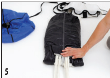
Reduce the canopy in preparation for d-bag placement.
