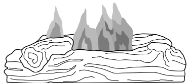
Figure 32 - Incorrect Burner Flame Pattern
