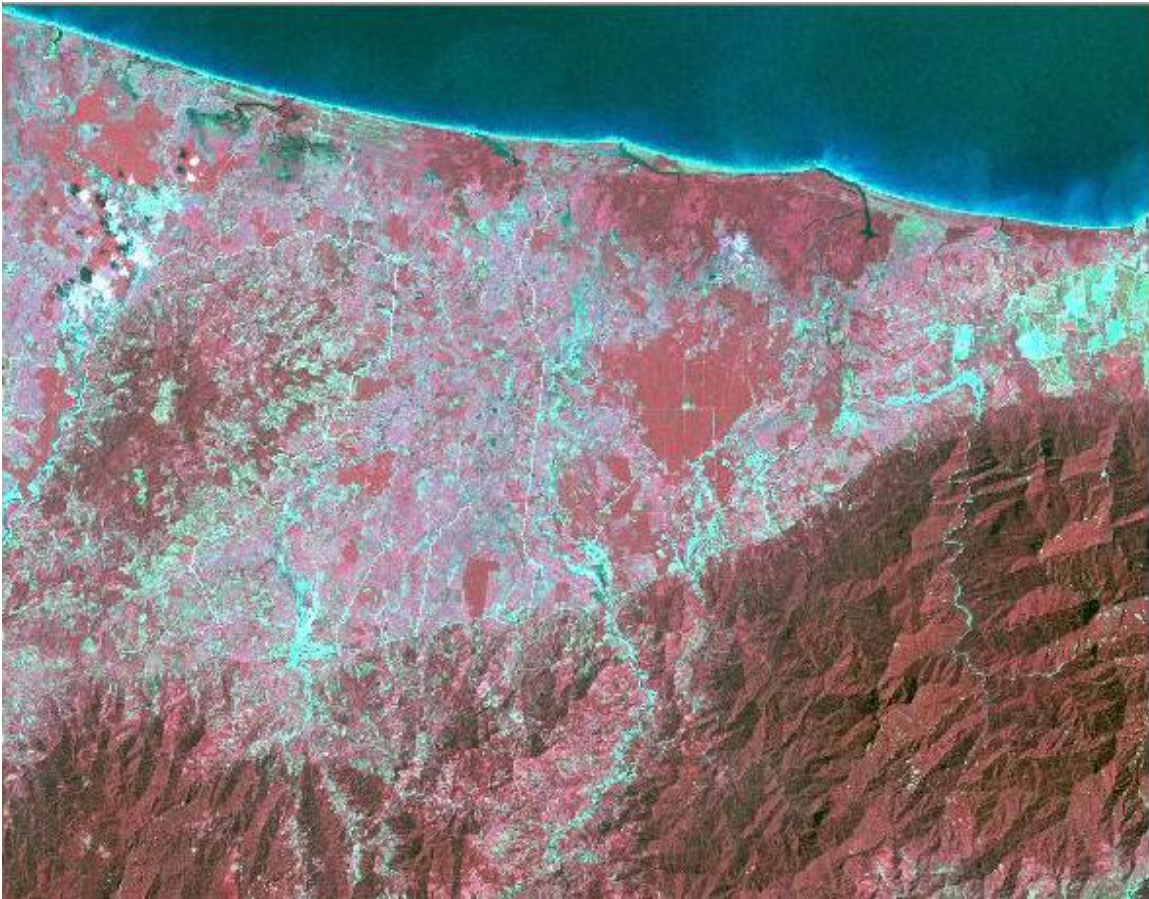
Northern Honduras from Enhanced Thematic Mapper on March 6, 2003 in near-infrared, red, and green wavelengths (bands 4,3,2).
