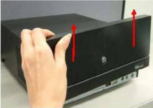
b. Lift the front cover up in the direction as shown by the arrows
