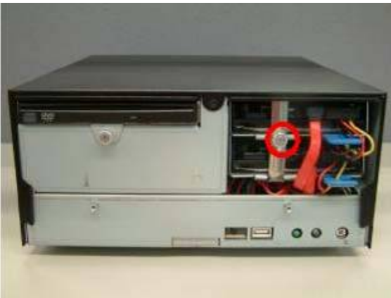
a. Loosen the thumb screw (1).
