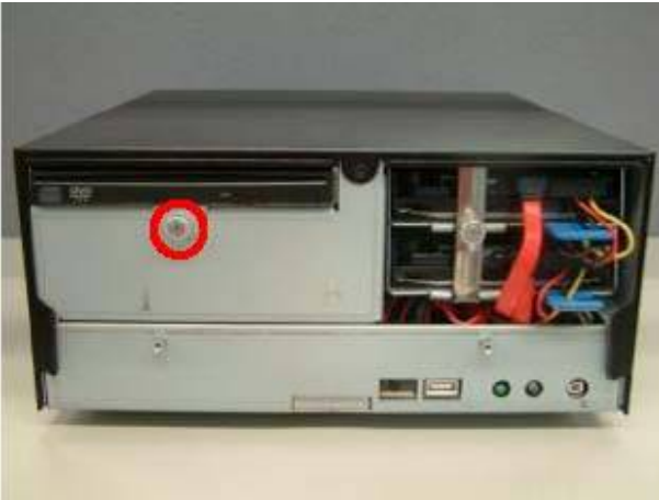
a. Loosen the thumb screw (1)
