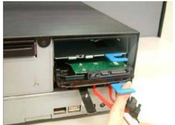
f. Repeat the step d. and e. to remove the other HDD.
