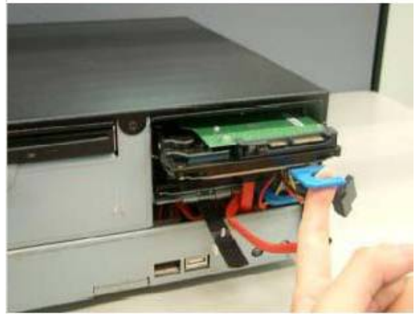
d. Use your finger to pull the HDD holder out.
