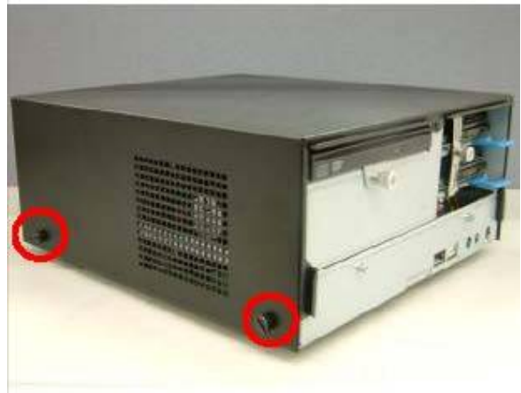
b. Loosen the thumb screws (4) (two from each side) to release the top cover from the system.
