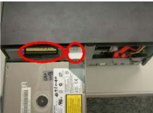
c. Disconnect the cables (2) to remove the DVD-ROM
