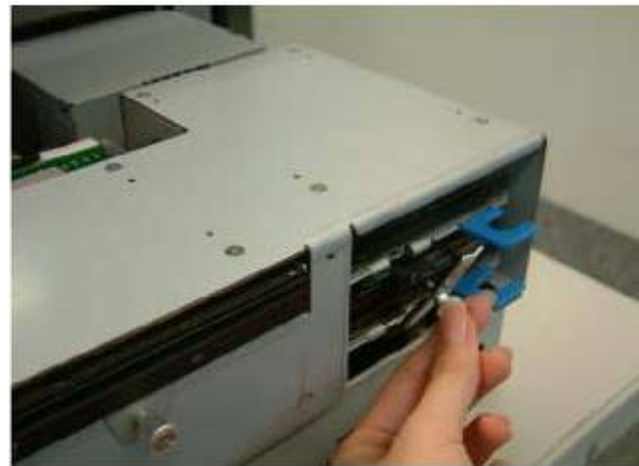
b. Loosen the locking bar (1).
