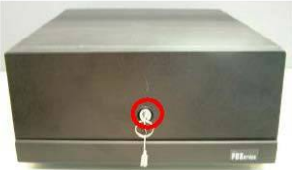
a. Use the key to unlock the front cover Remove the front cover
