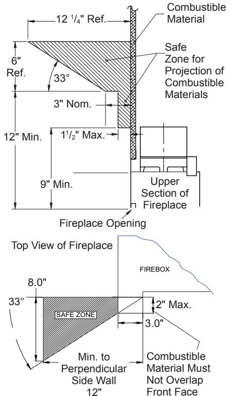
**Figure 4 - Mantel Clearances to Combustible Material**
