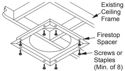
**Figure 10 - Firestop Spacer with Living Space Above Ceiling**
