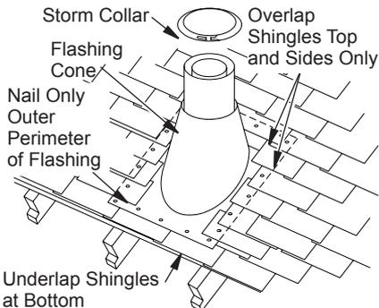
**Figure 13 - Flashing Installation**
