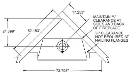
Figure 2 - Corner Installation
