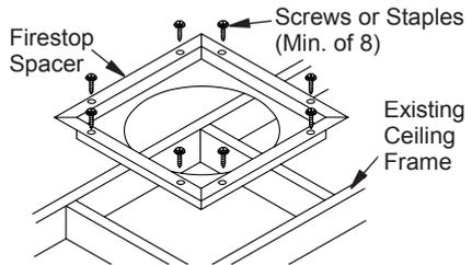
**Figure 11 - Firestop Spacer with Attic Space Above Ceiling**
