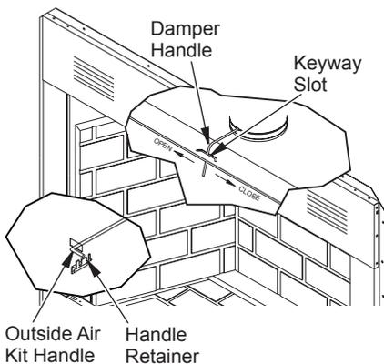
**Figure 22 - Damper and Air Kit Handle**
