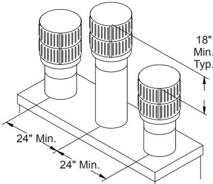
**Figure 16 - Multiple Chase Installation**
