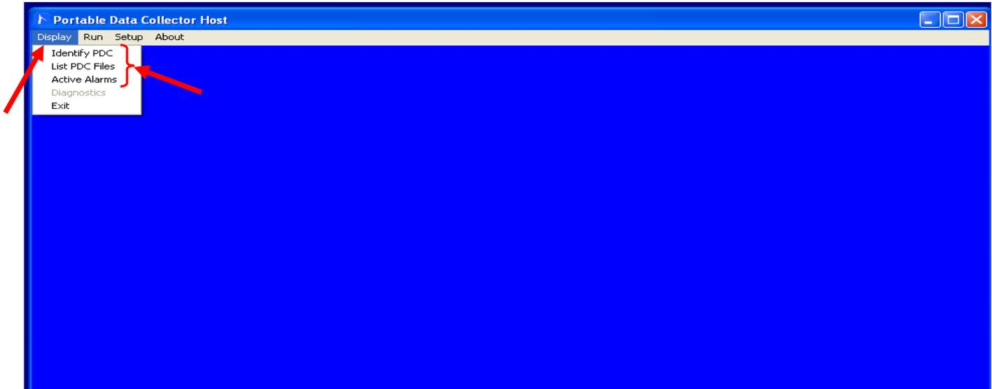
**Identify PDC:** Displays PDC Model & Firmware date. Also, viewing this screen confirms proper communication with the PDC).
