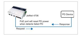
power to trigger remote PD cold start process. The connected PD can be automatically managed and reboot by JetNet 4706.
