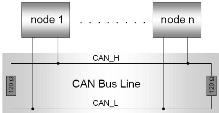
For easy installation, the LinMot DeviceNet controllers have built in termination resistors, which can be activated, if the LinMot controller is at the end of the bus line, and if there is no termination in the connector.
