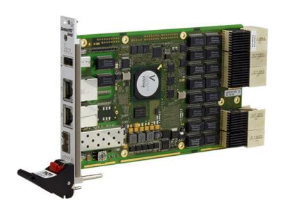
The G101 is a managed 3U flexible multiport Gigabit Switch, with a 29 GBit/s Switch matrix, implemented as a CompactPCI® Serial board. It occupies one system slot or one perpheral slot using a 4 HP front panel with two Gigabit Ethernet ports on RJ45 connectors and one 2.5 Gb SFP cage. Alternatively, the G101 can be supplied with three M12 connectors on the front panel.
