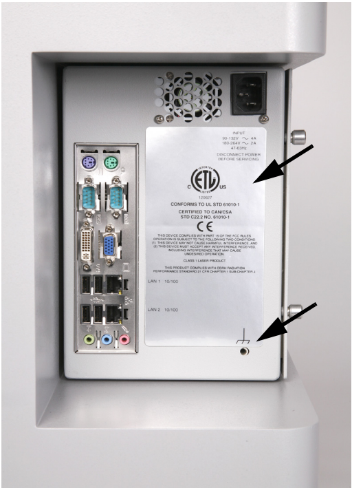
Figure 1-2. (a) Location of CDRH compliance label on the right side of the Odyssey Fc instrument. (b) Access hole for chassis ground.
