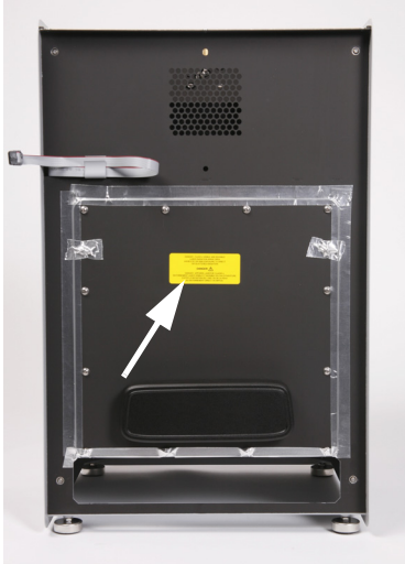
Figure 1-4. Location of class 4 laser warning label located on (a) the camera hood under the top panels of the Odyssey Fc instrument enclosure and (b) on the inner front access panel (do not open, no user-serviceable parts inside).
