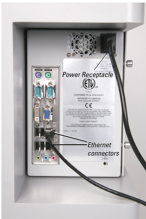
Figure 2-3. Close up of the Odyssey Fc control module showing the power receptacle and ethernet connectors (use only the supplied ethernet cable). All other connectors on this panel should not be used.
