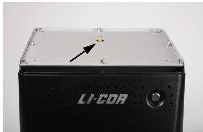
Figure 3-3. Odyssey Fc Imager with top panel removed. Location of the brass desiccant cap is indicated.
