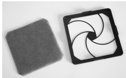
Figure 3-1. The foam fan filter on the back of the Odyssey Fc instrument is accessible for cleaning by removing the snap-on back cover.
