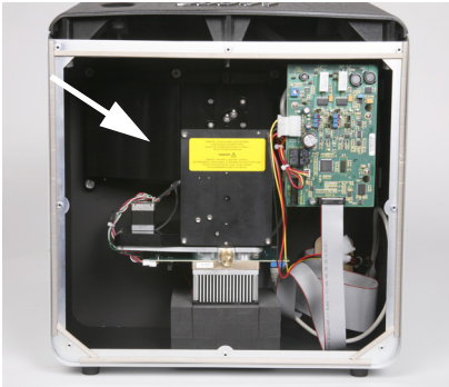
Figure 1-4. Location of class 4 laser warning label located on (a) the camera hood under the top panels of the Odyssey Fc instrument enclosure and (b) on the inner front access panel (do not open, no user-serviceable parts inside).
