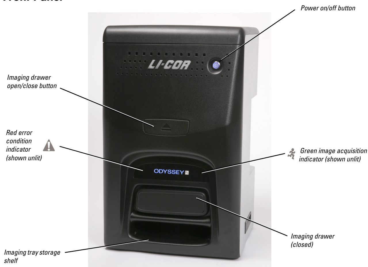
Figure 2-1. Front panel features and controls of the Odyssey Fc Imager.
