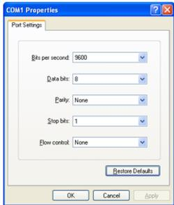
A standard serial data program such as HyperTerminal can be used to issue commands to the HDNet4P.
