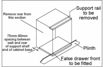
(Figure shows the ventilation and cut-out requirements for the installation of the appliance into a standard kitchen unit).
