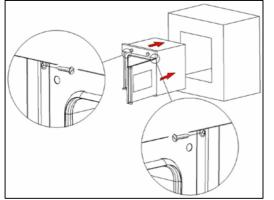
Ensure that the oven has been securely fixed into the housing unit. The fixing of the oven into the housing is made by using four screws. These should be screwed through the oven cabinet and into the housing unit.
