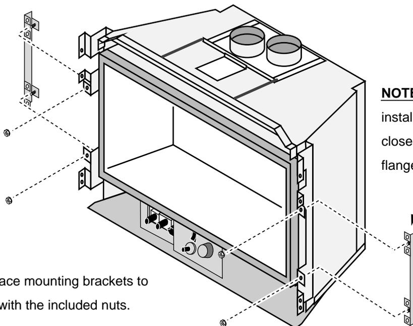
Install the face mounting brackets to the heater with the included nuts.
