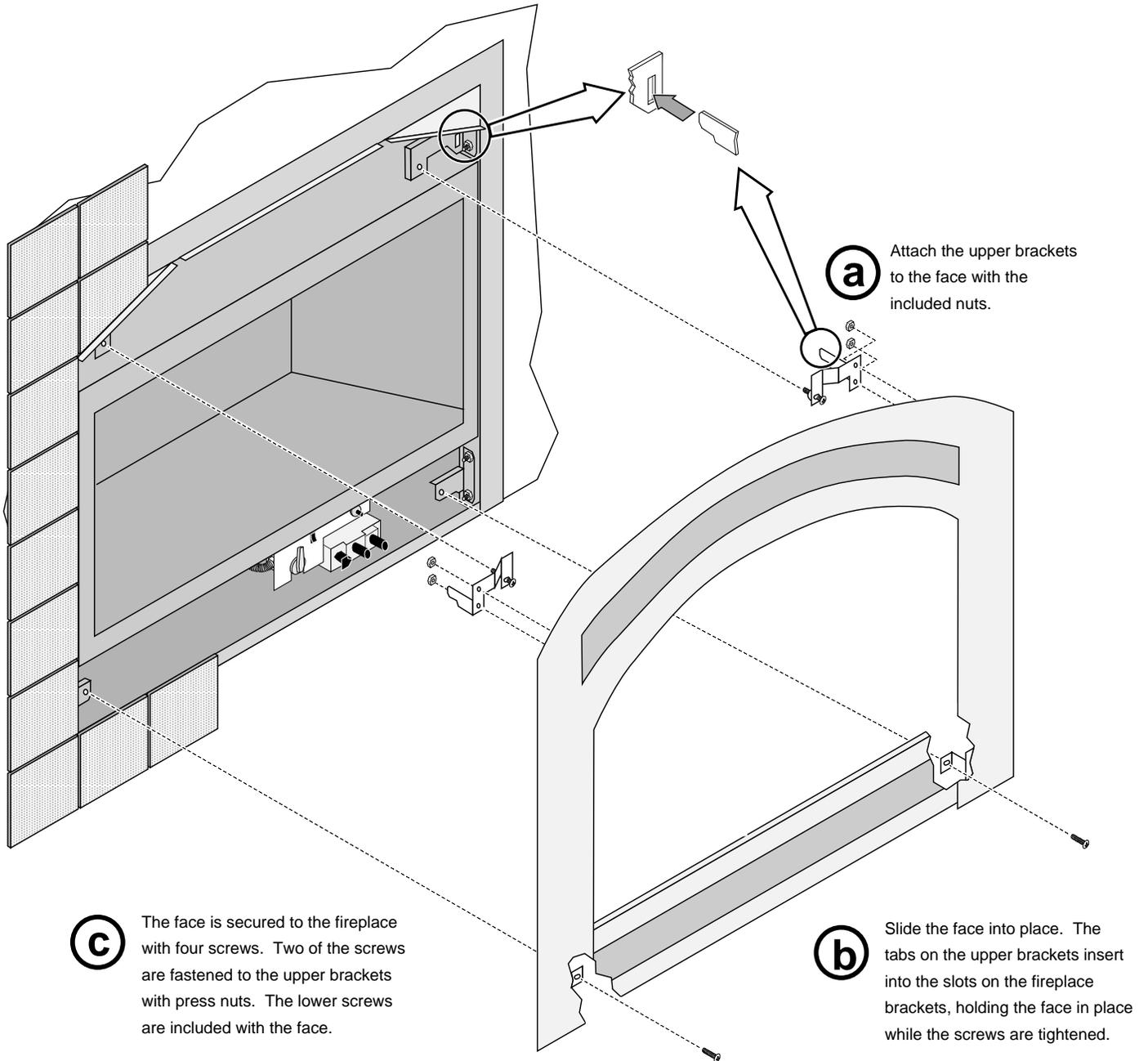
**c** The face is secured to the fireplace with four screws. Two of the screws are fastened to the upper brackets with press nuts. The lower screws are included with the face.
