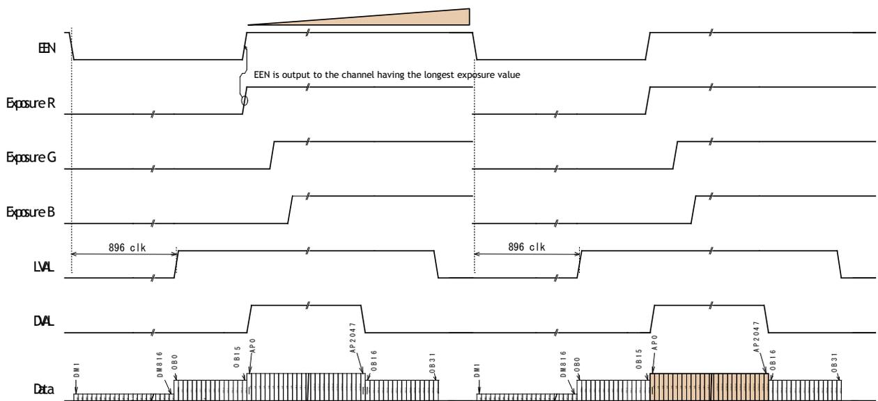
Fig.38 Shutter-select mode / Sub-sampling and Window / Internal
