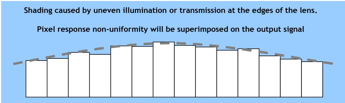
Fig.20 Shading correction
