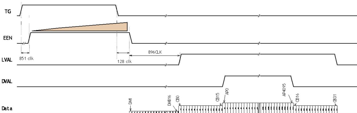
Fig. 42 Pulse Width Control mode
