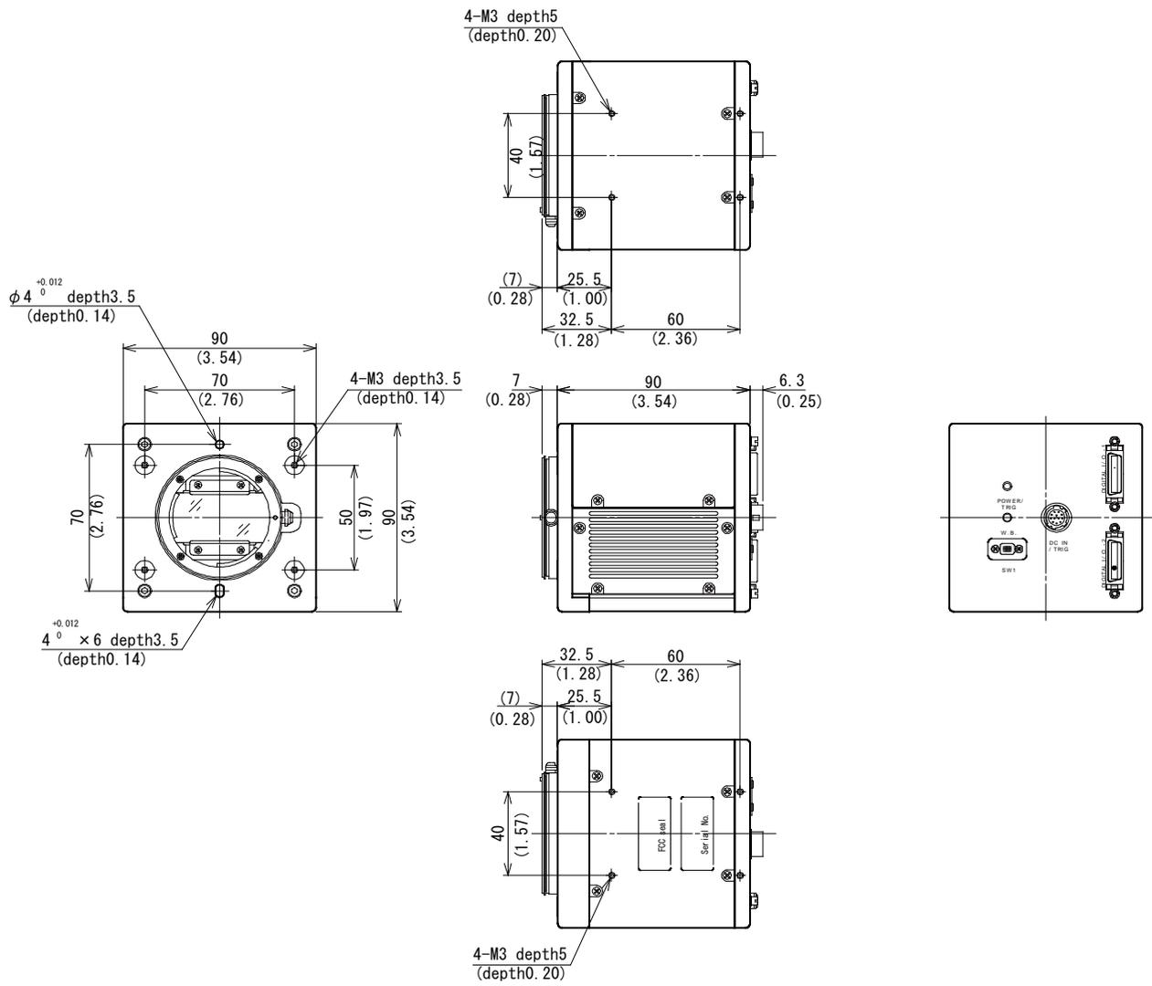
Outside size tolerance :  $\pm 0.3\text{mm}$
