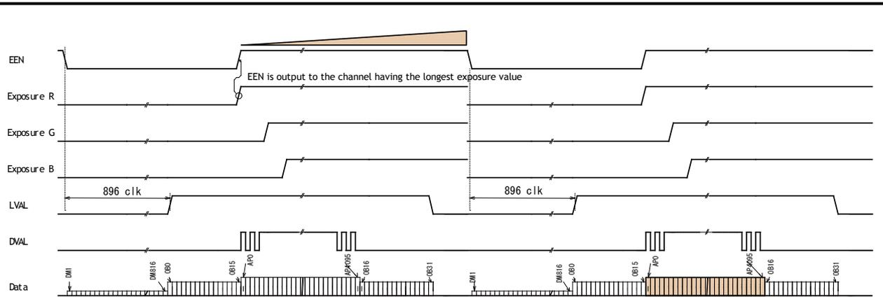
Fig.37 Shutter-select mode / Binning / Internal
