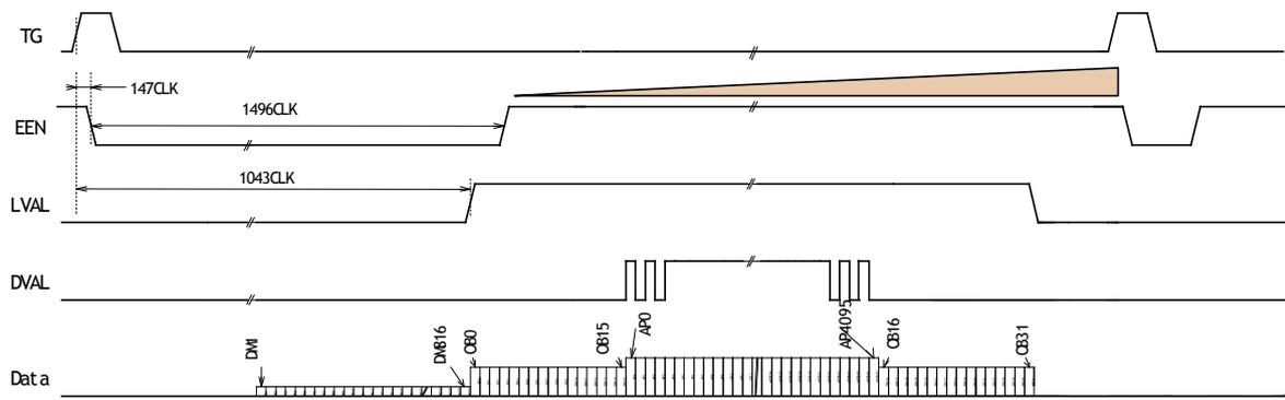
Fig. 34 No-shutter mode /Binning/ External
