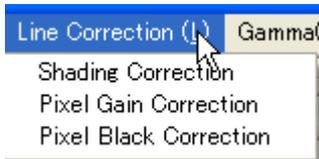
Click Line Correction menu and a drop-down menu will open. The setting window for shading, pixel gain and pixel black can be opened.
