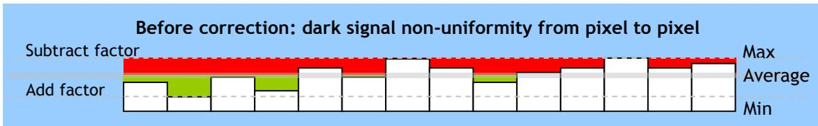
Fig.18 Conceptual drawing of DSNU correction
