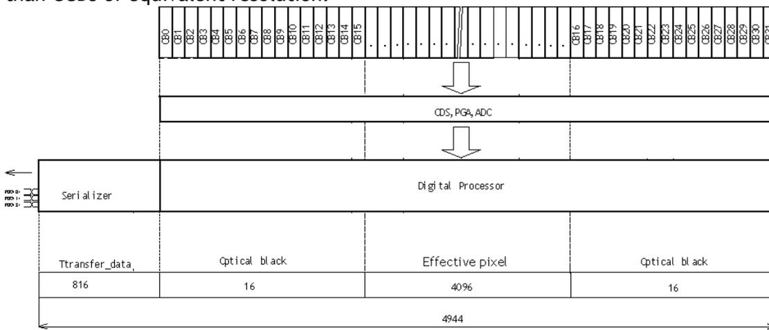
Note: Dummy pixels have photo diode.
