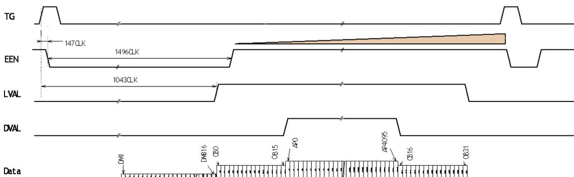
Fig. 33 No-shutter mode with external trigger
