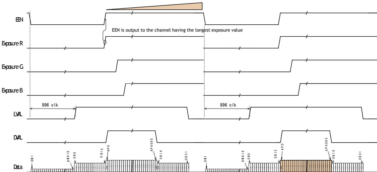
Fig. 36 Shutter-select mode with internal line rate generator (and individual exposure)
