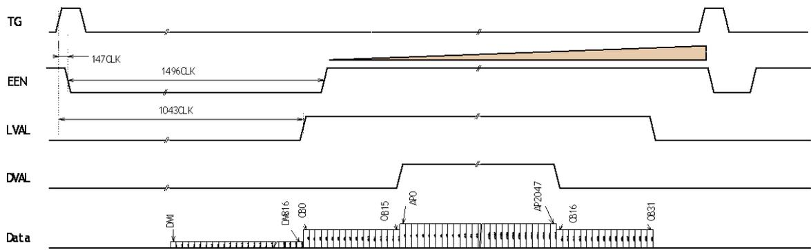
Fig. 35 No-shutter mode /Sub-sampling and Window/ External
