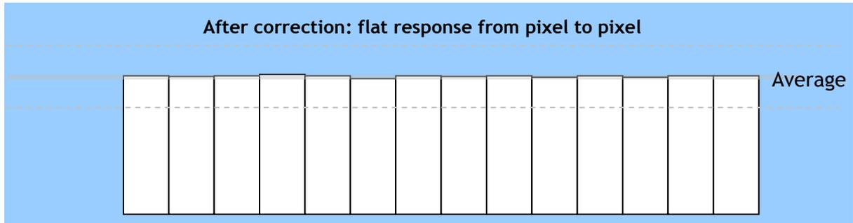
Fig.17 Conceptual drawing for PRNU correction (2)
