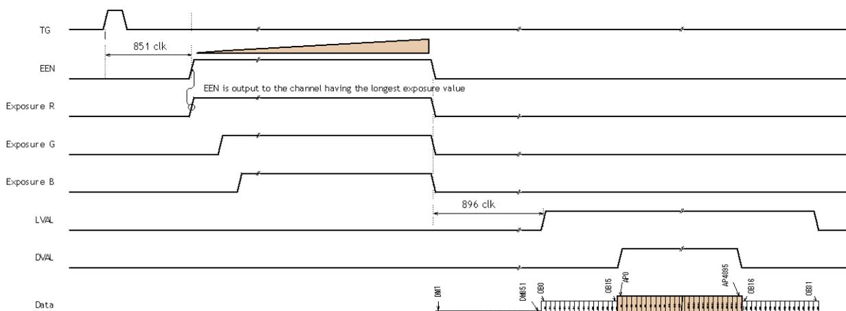
Fig. 39 Shutter-select mode with external trigger (and individual exposure)
