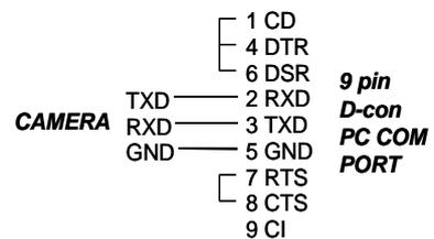
**Note:** Baud rate is available for 9600bps, 19200bps, 38400bps, 57600bps and 115200bps.
