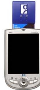
Make sure the card is right-side up. Push the card all the way in. If using a PC Card slot, first plug the card into a PC Card adapter.
