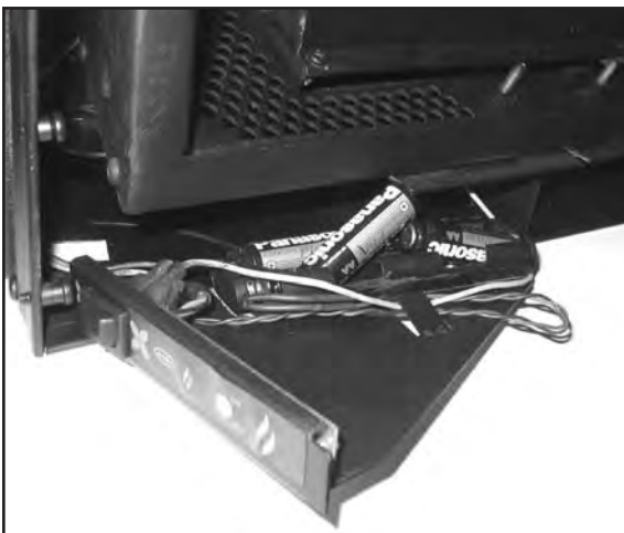
Figure 12: Control Panel & Battery Pack Bracket.
