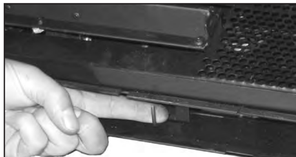
Figure 8: Adjusting the venturi air setting.
