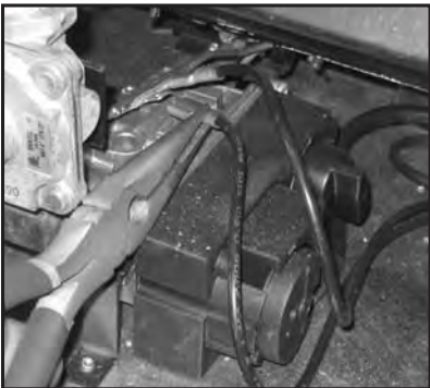
Figure 34: Remove Jumper From Thermocouple.
