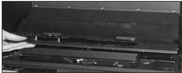
Figure 18: Removing Burner Tray.
