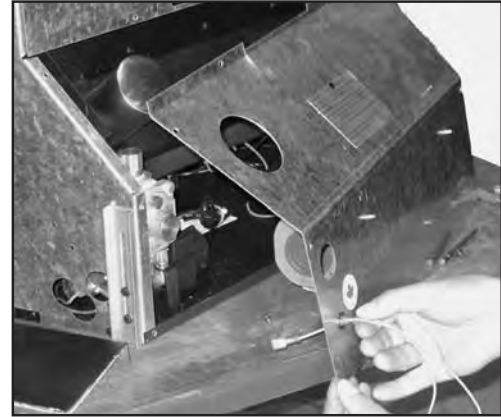
Figure 33: Spill Switch Wires Fed Through Back Panel.
