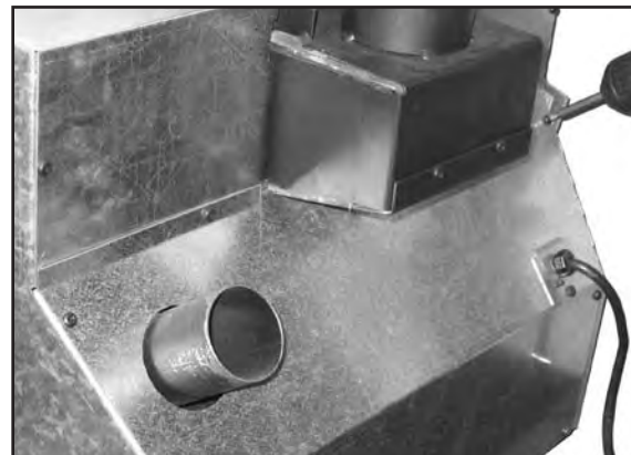
Figure 46: Removing/Installing Back Panel From Sonnet.
