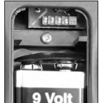
Figure 13: DIP Switch in Remote Handset Battery Compartment.
