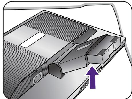
Orient and align the stand base socket with the end of the stand arm, then push them together until they click and lock into place.
