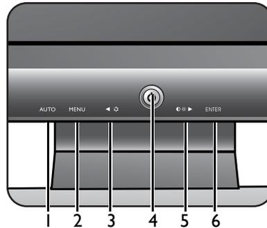
1. **AUTO**: Adjusts vertical position, phase, horizontal position and pixel clock automatically.
