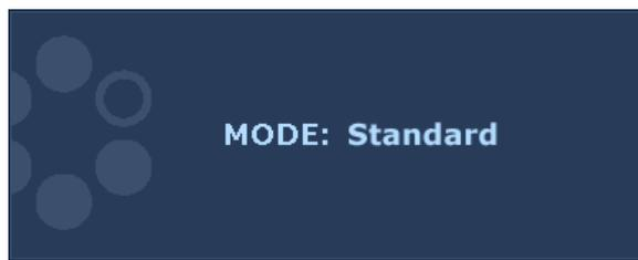
Press the **◀** key continually to switch between the 7 modes for the main window, including **Standard**, **Low Blue Light**, **Movie**, **Game**, **Photo**, **sRGB**, and **Eco**. The setting will take effect immediately.
