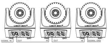
The communicate cable is 2-pin shielded cable  $75\Omega$
