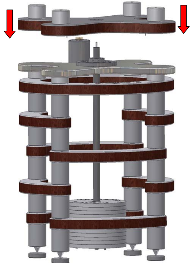
Pic. 9: Removing the wooden spacers
