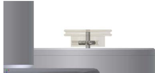
Pic. 20: Setting the motor pulley
