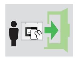
Display module integration. Access control is also available in Welcome M. Proximity reader is integrated in LCD module for convenient access for authorized users. The in-built Wiegand output make it easier to integrate into a third party controller.
