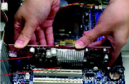
5. Replace the screw to fasten the card in place, and replace the computer cover.
