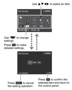
Most functions are set from the menus. The functions that can be set on the control panel can also be set from the menus.
