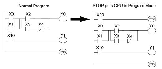
In the example shown above, you could trigger X20 which would execute the STOP instruction. The CPU would enter Program Mode and all outputs would be turned off.
