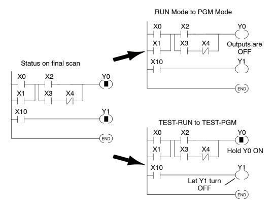
Before you decide that Test Mode is the perfect choice, remember the DL350 CPU also allows you to edit the program during Run Mode. The primary difference between the Test Modes and the Run Time Edit feature is you do not have to configure each individual I/O point to hold the output status. When you use Run Time Edits, the CPU automatically maintains all outputs in their current states while the program is being updated.
