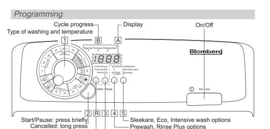
delay start functions Apart from the «On/Off» button (Ein/Aus), all the buttons are sensitive and therefore do not remain depressed.
