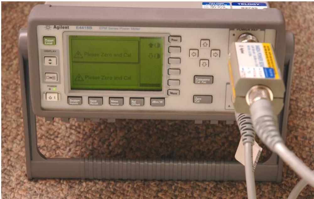
**Figure 4.1** Calibrating the Agilent power sensor
