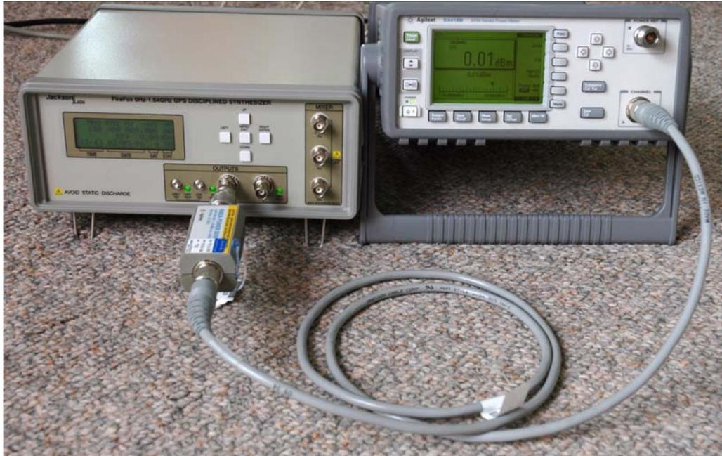
**Figure 4.2** Connecting the power sensor to the FireFox RF output
