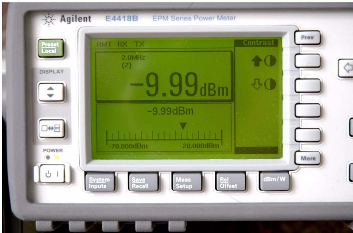
**Figure 4.8 Agilent power meter display during calibration**
