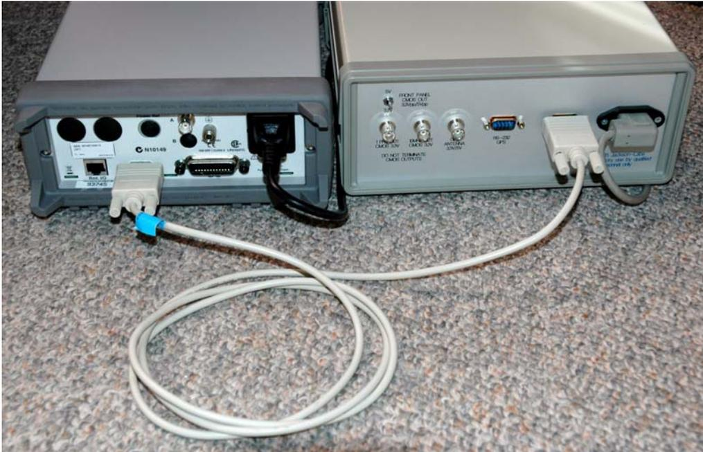
**Figure 4.4 Power Meter Serial Communication connection**
