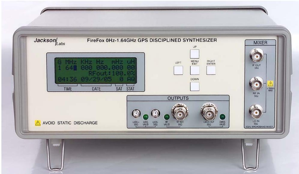
Figure 1.1 FireFox Desktop Unit Front Panel
