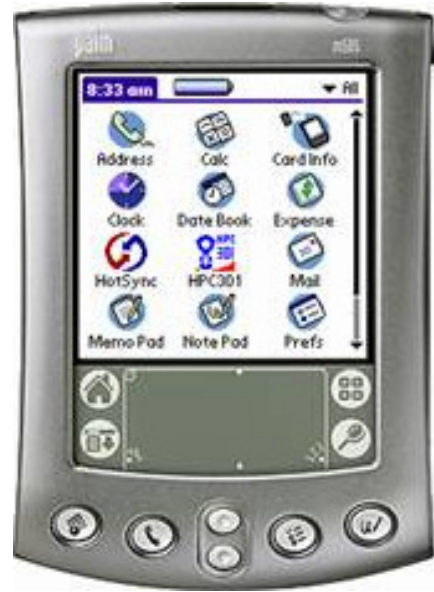
Figure 3.1 - Smar's HPC301 Hand-Held Terminal
