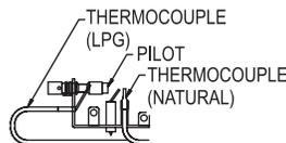
in for about one (1) minute after the pilot is lit. Release knob and it will pop back up. Pilot should remain lit. If it goes out, repeat steps 4 through 8.
