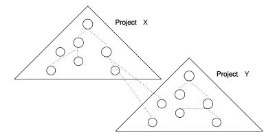
As one can see, some of the cells in projects X and Y are defined hierarchically, instantiating local cells. Project X however also contains cells which instantiate cells from project Y. These remote cells have been imported previously into project X, before instantiating (= referring) them within this project.
