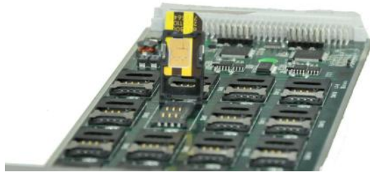
Fig: Inserting SIM in SIM Server card.
