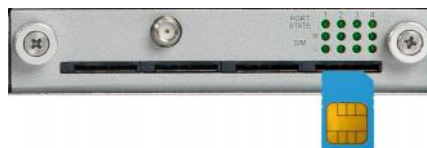
Fig: Inserting SIM in Cellular card.
