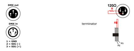
How to turn the controller line from 3-pins into 5-pins (plug and socket).
