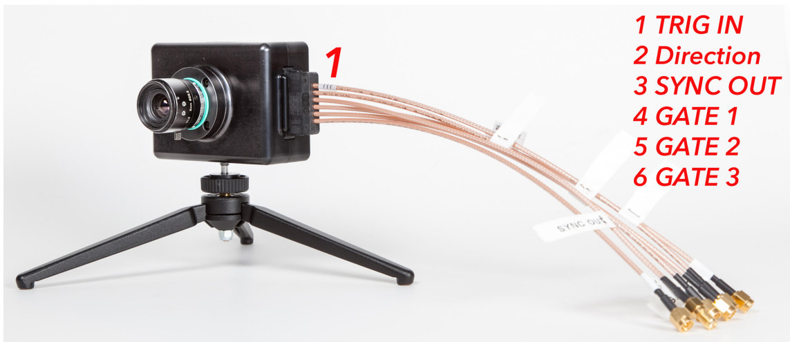
Figure 4. Camera with the cable adapter and the SMA output description.
