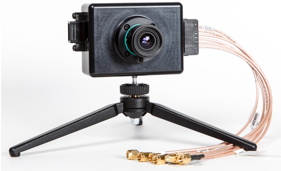
Figure 1. SPC 3 : Single photon Counting Camera.
