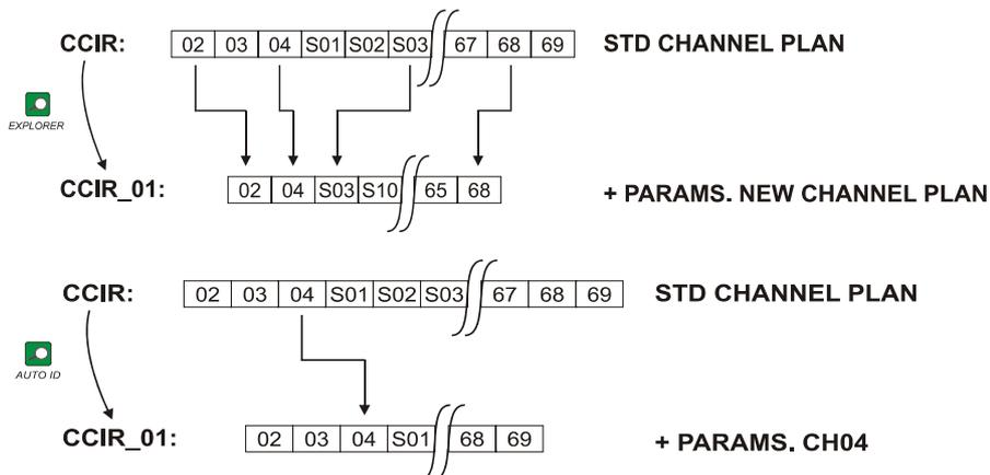
**Figure 9.-** New channel plan generation process.
