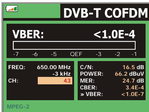
Figure 22.- Screen of BER measurement (COFDM signals). VBER.
