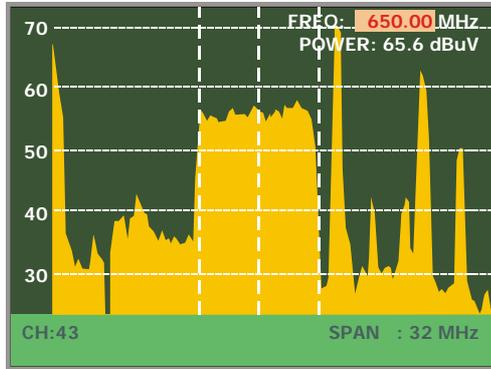
**Figure 27.-** Spectrum analyser mode.
