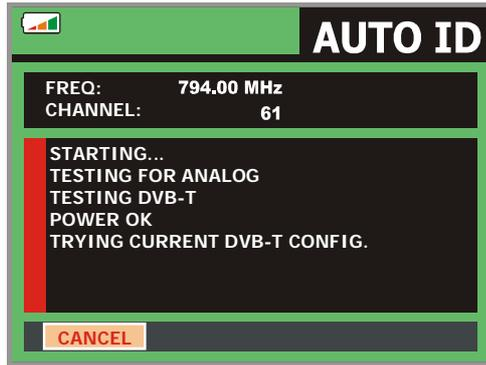
**Figure 8.-** Signal automatic identification screen. **AUTO ID.**
