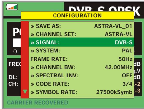
Figure 13.- Screen of measurement configuration (QPSK signals).
