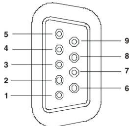
**Figure 32.-** RS-232C connector. External view.
