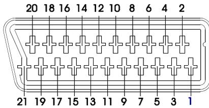
**Figure 33.-** Scart socket (external view).
