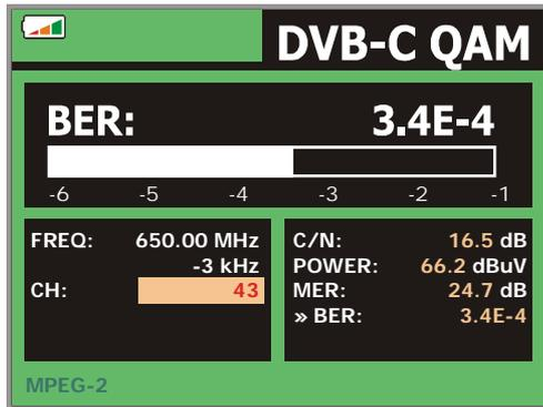
Figure 18.- Screen of **BER** measurement of **QAM** signals.
