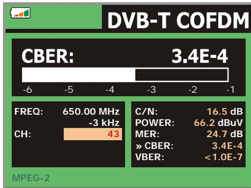
Figure 20.- Screen of CBER measurement (COFDM signals).
