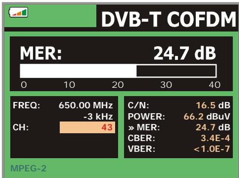
Figure 26.- Screen of MER measurement of DVB-T (COFDM) signals.
