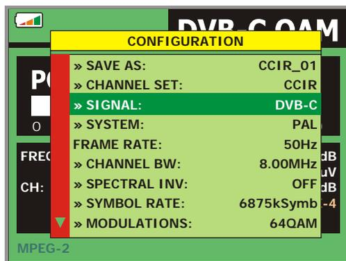
Figure 11.- Screen of measurement configuration (QAM signals).
