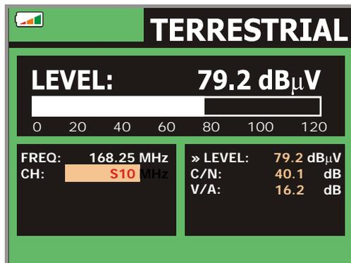
**Figure 14.-** Analogue signal level measurement in terrestrial band.
