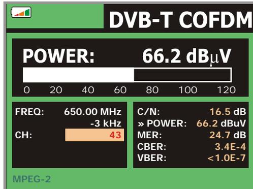
Figure 17.- Digital channel power measurement.
