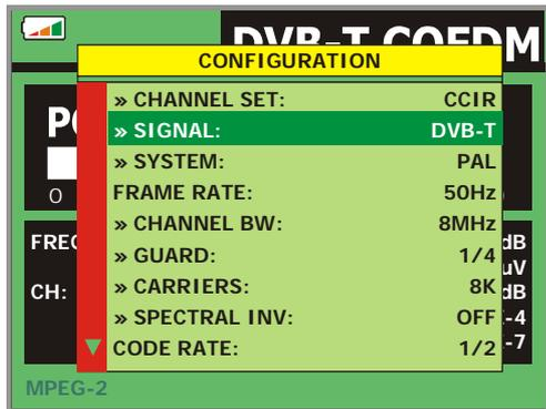
Figure 12.- Screen of measurement configuration (COFDM signals).
