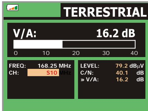
Figure 15.- Measurement of the video/audio rate
