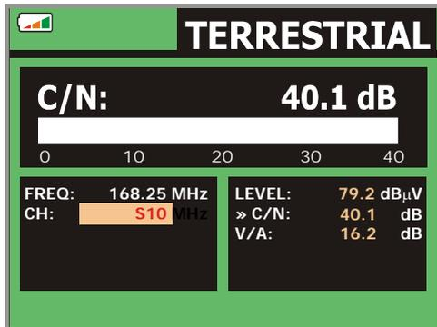
**Figure 16.-** Carrier-to-noise ratio measurement (C/N).
