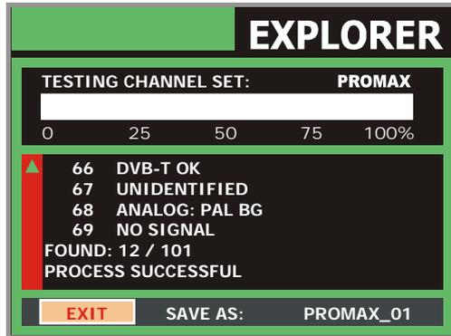
Figure 10.- Spectrum exploration screen. **EXPLORER**.
