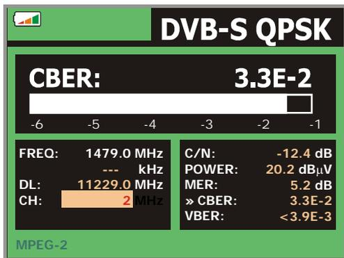
Figure 23.- Screen of CBER measurement (QPSK signals).
