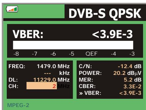
Figure 25.- Screen of VBER measurement (QPSK signals).
