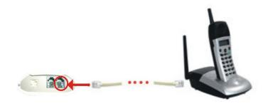
**STEP 5:** Connect a telephone cable between the USB GATEWAY **line** jack and a wall jack as shown below. Note that this is only required for making regular phone calls or for forwarding Skype calls to your mobile (or other off-site) phone or for toll bypass applications.
