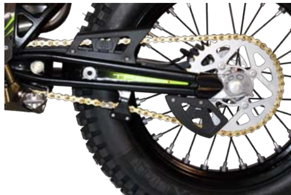
Chain drive and tension adjuster springs
