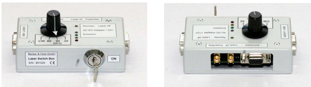
Fig. 3: Laser switch and connection box
