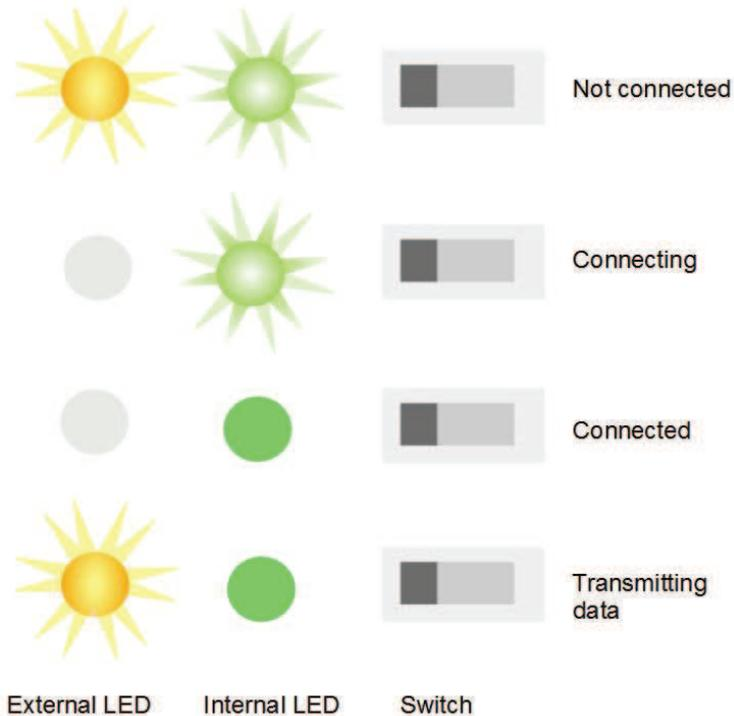
**Figure 11: Visualization of the connection state with LEDs**
