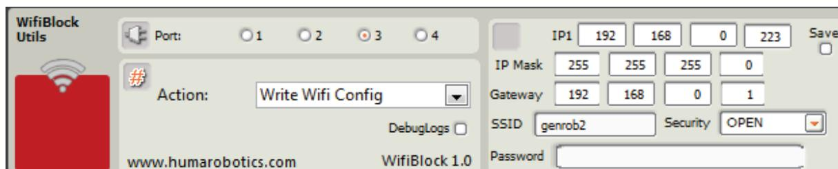
**Figure 9: Configuration panel for the WifiBlock**
