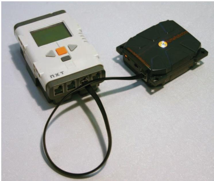
Figure 4: Connection between the Lego Mindstorm Brick and the WifiBlock
