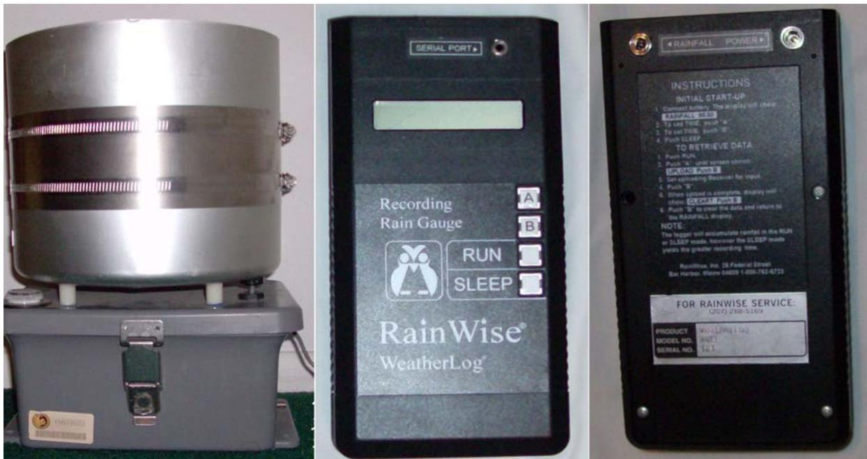
Figure 4. RainWise rain gauge (first) and logger (middle and right).
