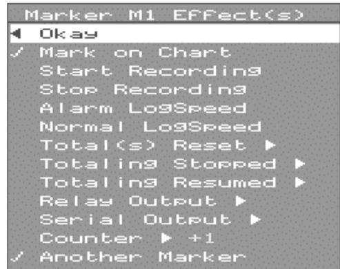
When the Counter is enabled, the value of the Counter can be incorporated in the description of the marker by entering an exclamation mark in the description text. For example, if you want the counter value to represent a batch number, enter the text **BATCH NO.!** in the description field of the marker. The counter value will automatically be inserted in place of the exclamation mark every time that marker is set.
