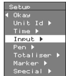
Selecting **Input** from the Setup menu generates the inputs option list. Depending on the model, only the number of analogue channels available can be selected starting with Input 1.
