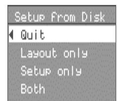
When Setup from disk is selected only files with the **.OPC** extension are loaded.
