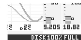
When 90% of the disk space is used up, the Disk space status changes colour from green to red. This indicates that disk space is running out and a new recording on a new disk should be started.
