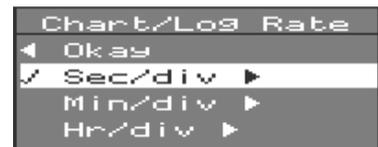
Selecting **Log Speed** brings up an options menu offering three ranges of chart speed, with the current range indicated by a ✓. The chart speed is the time period between each vertical division of the chart
