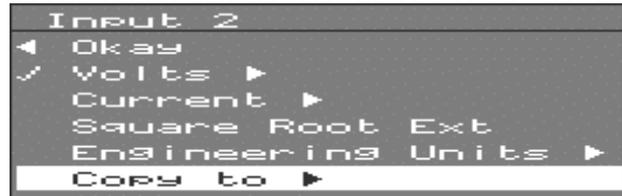
In this example Inputs 3, 4, and 6 will be configured in the same way as Input 2.
