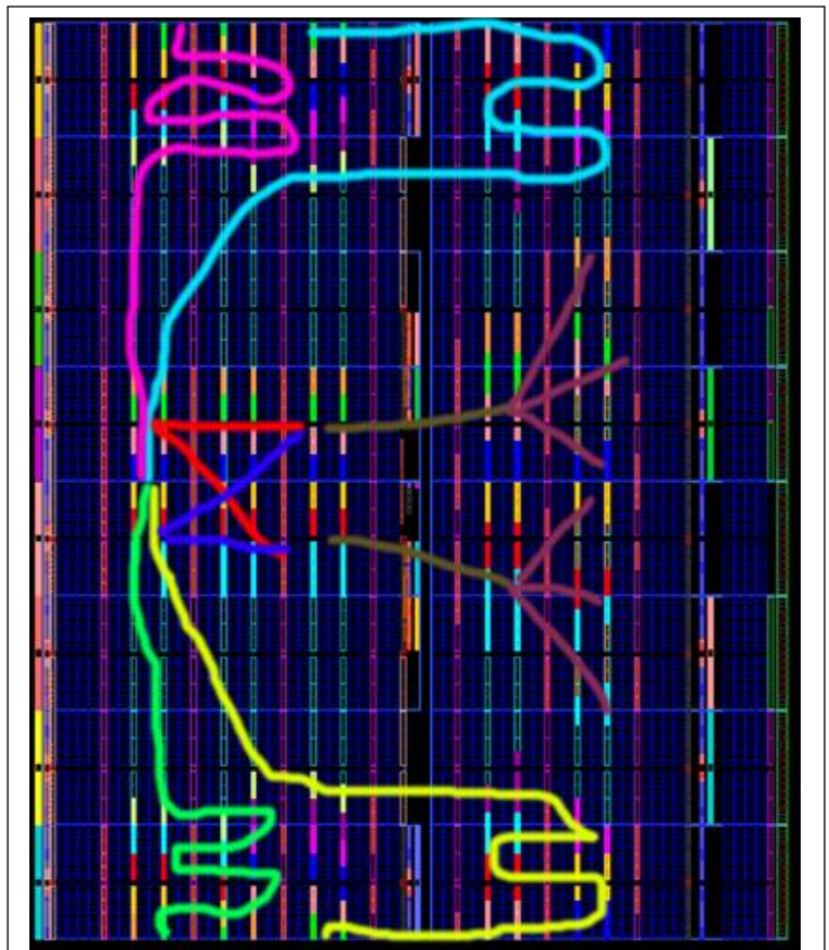
Actual Spectrometer Floorplan, data-paths annotated. Planning datapaths in advance is crucial.
