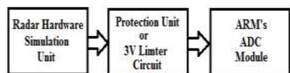
Figure 1 Hardware block diagram of the radar signal pretreatment part.
