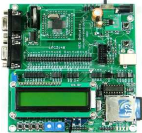
Figure 6 ARM7 LPC2148 development board
