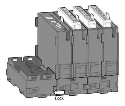
Step 5: Insert the upper case of APAX-5343E back on its backplane. Use tongueand-groove slots to move the upper case.
