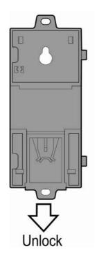
Step 2: Hang the APAX-5002 backplane onto the screw on the wall (panel). The screw for APAX-5002 to hang should be special-designed. We have provided it in accessory.
