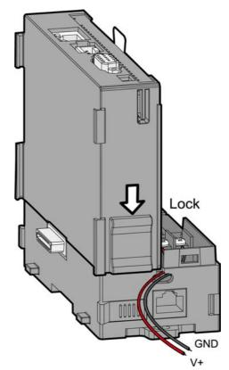
Step 4: Insert another APAX-5000 I/O module on the same APAX-5002 backplane. Use tongue-and-groove slots to move the module.
