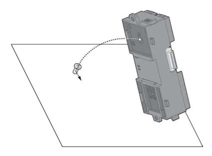
Step 3: Mount the first APAX-5002 backplane to the wall (panel) using two standard M4 or #8 panhead screws. We also provide the two screws in accessory.
