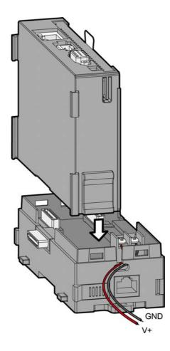
Step 3: Lock APAX-5522PE to the APAX-5002 backplane by pulling down the module locks on two sides.
