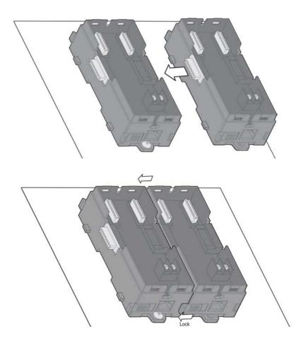
Step 5: Mount that APAX-5002 backplane to the wall (panel) using two standard M4 or #8 panhead screws.
