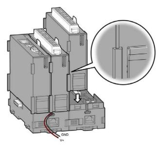
Step 9: Lock that APAX-5000 I/O module to the second APAX-5002 backplane by pulling down the module locks, similar as step 5.
