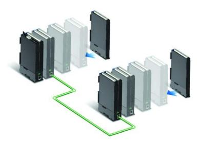
APAX-5522PE supports the redundant function. To leverage this functionality, two CPU modules (controllers), with the same control program, are installed in one system. After both controllers are enabled to have backup function, the APAX-5000 system will automatically delegate one of the two controllers as the master controller.
