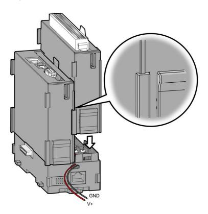
Step 5: Lock that APAX-5000 I/O module to the APAX-5002 backplane by pulling down the module locks on two sides.
