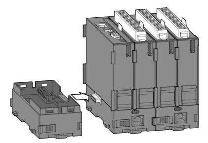
Step 4: Lock the stacked APAX-5343E backplane to the APAX-5002 backplane by the backplane locks on the APAX-5002 backplane.
