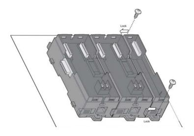
Step 7: Insert APAX-5522PE and all necessary APAX-5000 I/O modules to the backplanes. (Similar to Step 2, Step 4 and Step 8 in section 3.1.1)
