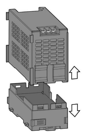
Step 3: Stack the backplane of APAX-5343E to the left side of the first APAX-5002 backplane in the system.
