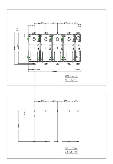
Below are the procedures for the wall (panel) mounting.
