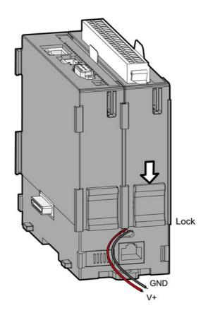
Step 6: If you need more than one APAX-5000 I/O module, stack another APAX-5002 backplane to the original APAX-5002 backplane.
