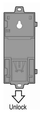
Step 2: Attach the APAX-5002 backplane on the DIN rail.
