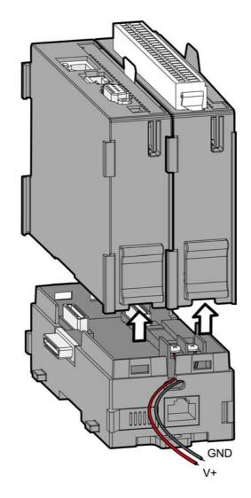
Repeat Steps 1 ~ 2 for the APAX-5000 I/O modules disassembly.
