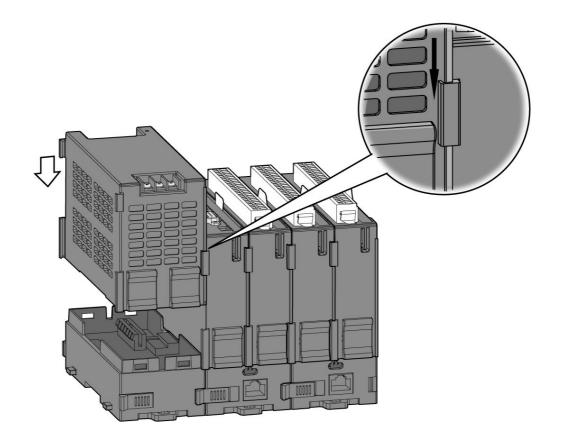
Step 6: Lock the upper case of APAX-5343E to its backplane by pulling down the module locks on the upper case. Connect AC power code to the power connectors on the upper case of APAX-5343E. Then the whole system is powered-on.
