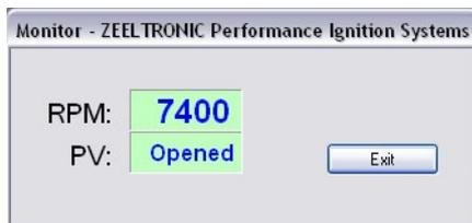
⇒ Monitor show engine revolution and PV position.
