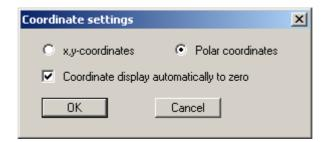
the coordinates are displayed in the status bar in polar coordinates. In addition, these coordinates are reset to zero at each mouse click. This means that the current diameter of the circle is always displayed.
