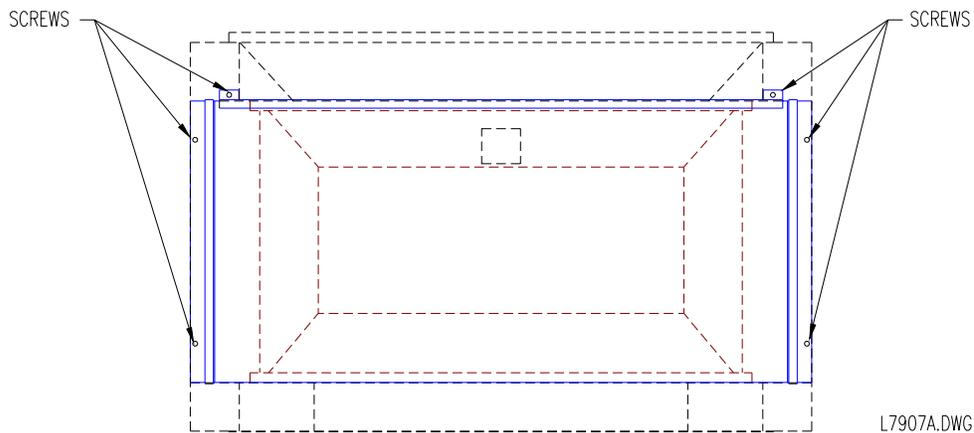
\* To remove the glass front, unscrew the six screws holding it in place as shown.
