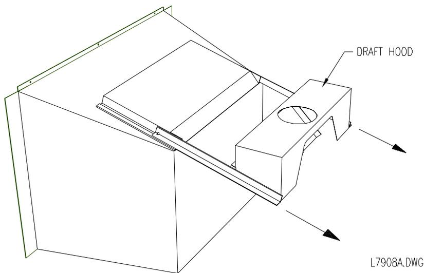
5. Move the ULTRA FLAME to the desired position and level the appliance using the two bolts located in the back corners. Mark the location for the gas inlet pipe. ( We suggest using the hole in the back of the ULTRA FLAME for ease of connection. )
