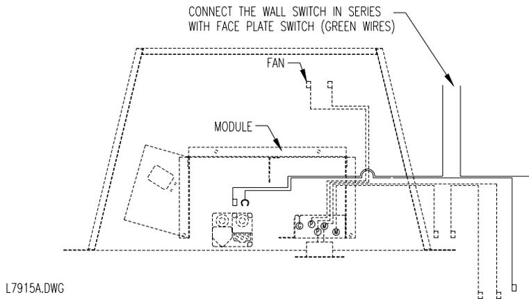
19. If you want to turn the main burner ON and OFF using a wireless remote control, install the remote control module apart from the gas valve and as close to the front as possible. Connect the wires as shown.
